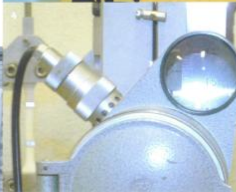
1 Julien Lebranchu calibrating the camera to measure the creep on small plastic pieces put under different weight constraints 2 From left to right, the team involved in the CreepMan project: Daniel Ayglon, Julien Lebranchu and Alexandre Antonijevic.
