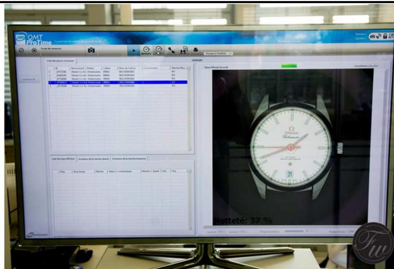
The accuracy of a watch is being measured and monitored using photo equipment and by 'scanning' the positions of the hands.
